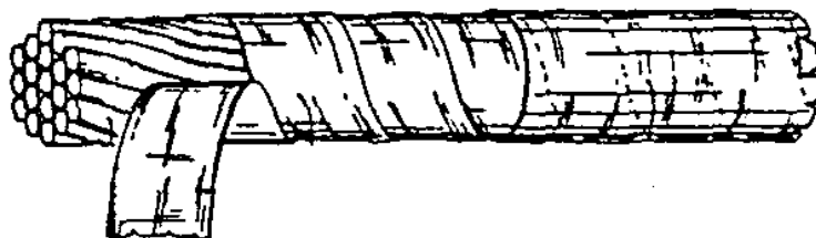
Figure1: Example of implementation of EIS by taping technology
